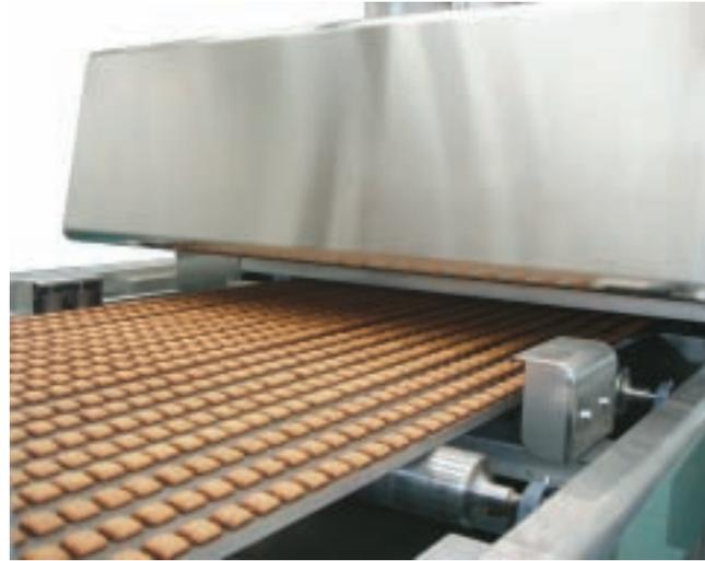
Sandvik solid and perforated steel belts are the ideal medium for conveying all kinds of baked products. The tough, hard wearing surface guarantees product quality and gives bakers years of excellent and predictable service with a belt that stays flat, keeps its shape and maximises production output.
