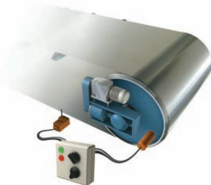
*Above illustration shows an active steel belt tracking control using electromechanical actuation controlled by a programmable relay. This automatic tracking device is normally used in bake oven lines mounted at the axle neck on the head end drum.*
